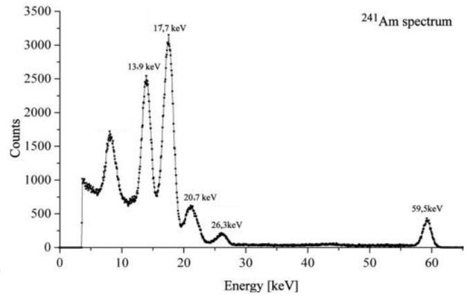
*Left: Americium 241 spectrum showing the characteristic peaks measured with a test CCD in the test set-up at IFAE.
