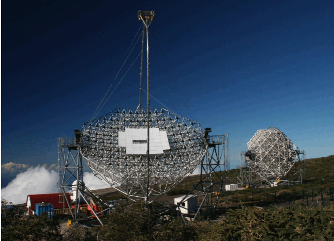
*A picture of MAGIC-II after mounting 20% of its mirrors in summer 2007. In the background, the electronics control building and the first MAGIC telescope.*
