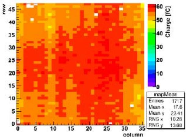
*MicroMega gain uniformity obtained with the Test Bench at CERN. The observed non-uniformity is of the order of 10% and it is explained from the capacitance of the readout lines.*
