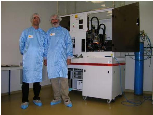
*Shown a photo of the flip-chip machine FC150 during test and calibration at Suss Microtec site in St. Jeoire, France.*
