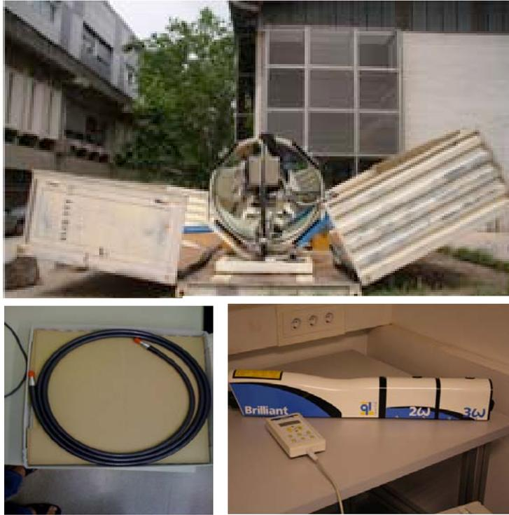
*Fig. 3 Some of the elements of the Raman LIDAR being built at IFAE for CTA: the CLUE container plus a 1.8 meter diameter telescope, the QUANTEC Brilliant Nd-YAG laser of 360mJ/pulse @ 1064 nm with a frequency tripler, and the LUMATEC liquid lightguide series 300 with 8mm diameter and 3200mm length.*
