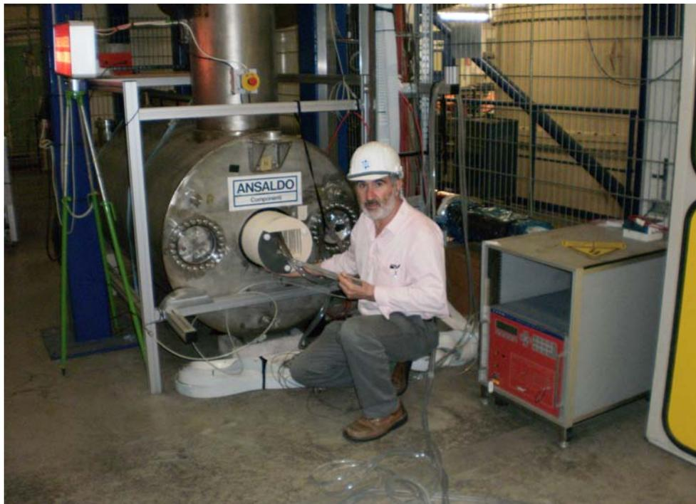
Fig. 4: Insertion of a Medipix 2 CdTe sensor in a 4 Tesla magnetic in DESY, Hamburg.
