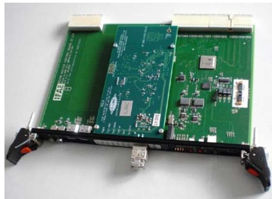
*Fig. 2: One of the Master Control Board (MCB) cards for the DECam produced at IFAE in 2010.*
