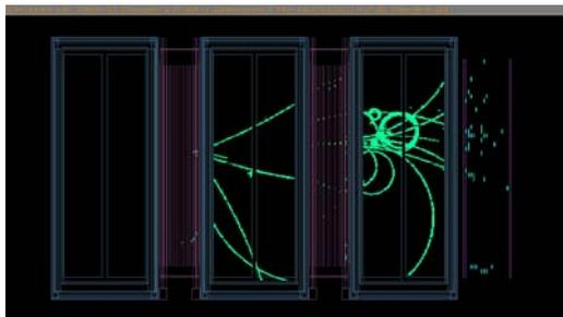
Fig.4.Event display showing a multi-track interaction in the Fine-Grain Detector (FGD) and the tracks detected in the TPC volumes.
