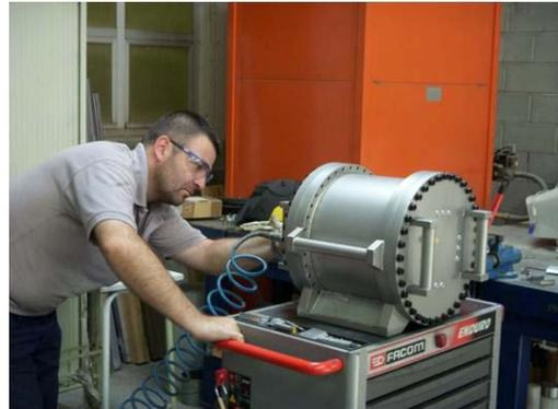
Fig. 8. The pressure vessel of the 30 APD chamber.
