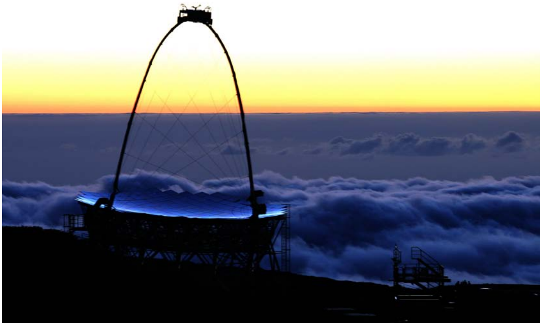
Fig 1 (copyright R. Wagner): The second MAGIC telescope points at zenith shortly after sunset. The new 1039 photomultiplier camera is installed at a focal distance of 17 meter from the 17 meter diameter mirror dish. The MAGIC telescopes are equipped with the largest optical reflectors in the world. These huge photon collectors enable the telescopes to detect \gamma -rays in the energy band from 25 GeV to a few tens of TeV.
