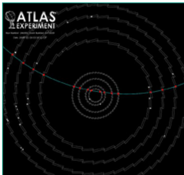
**Fig. 1: A cosmic ray is shown passing through the IBL, the newly installed pixel layer of the ATLAS detector, in the presence of a solenoidal magnetic field.**
