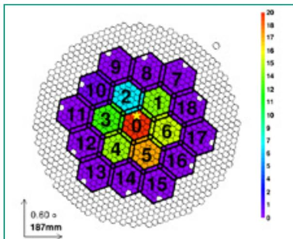
**Fig. 2:** The color scale shows the spatial distribution of triggering macro-cells in one of the MAGIC cameras for events triggering macro-cell #0 in the other MAGIC camera. Thin lines represent the camera pixels. Macro-cells are defined as groups of pixels whose combined signal is used to issue a level-0 trigger, and are depicted in the plot by thick lines and labeled with numbers. 99.4% of the macro-cells triggering in one telescope are within the first ring around macro-cell #0.
