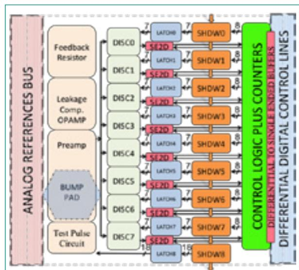
**Fig 6.** ERICA single pixel block diagram
