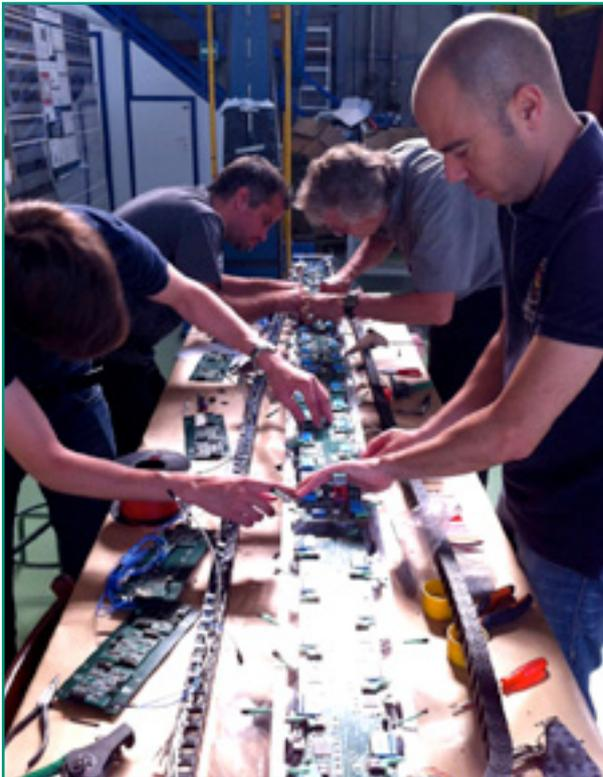
Fig. 2: Mounting front-end electronics on the mechanical structure build at IFAE
