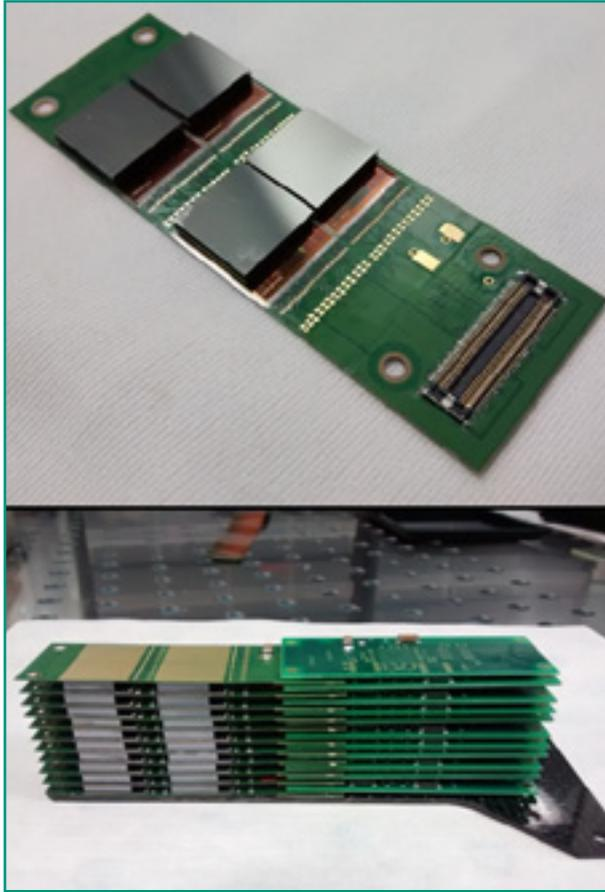
**Fig 5:** On the top one can see a single layer of the VIP module with 4 VIP sensors mounted on 255µm thick PCB. On the bottom one can see the VIP module, a stack of 10 layers, with the total of 40 VIP sensors. The VIP module has 4000 voxel sensors, and each voxel has the size of 1mm x 1mm x 2mm
