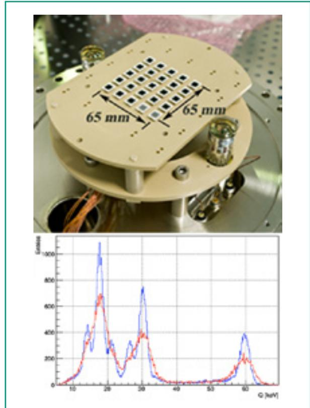
**Fig. 9: (Top) APD readout plane (Bottom) measured spectrum before (red) and after applying the inter-calibration method (blue). The best result was 5.2% FWHM at 59.5 keV.**
