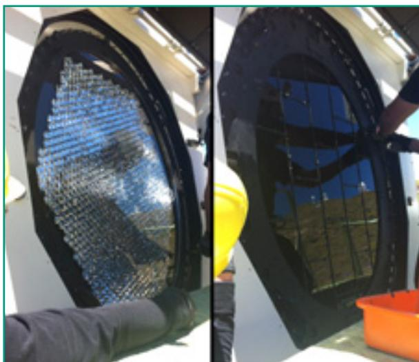
**Fig. 3:** The MAGIC PMT camera before (left) and after (right) the installation of the UV-pass filters. MAGIC PMTs have low gain, which allows observation under moderate moonlight. Thanks to the filters MAGIC is now able to observe in every Moon phase and as close as  $\sim 4$  degrees away from the Moon.
