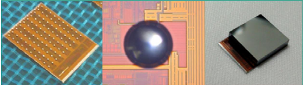
Fig 4: On the left one can see a single VIP chip (10mm x 13mm) and the UBM (gold) deposited at the input of each pixel. In the center one can see the 250um BiSn solder ball deposited on one of the input pixels. On the right one can see the VIP "sensor" which has a 10mm x 10mm x 2mm pixel CdTe detector bonded to a VIP chip via bump-bonding process.
