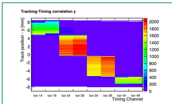
Fig. 3: The spatial correlation of the tracks in the pixel detector and the timing bars (placed directly behind the tracker) indicate the successful integration of the AFP detector prototype.
