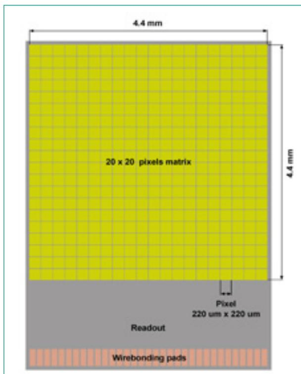
Fig. 7: Schematic layout of the ERICA chip. It has an array of 20x20 pixels with total size =  $4.4\text{mm} \times 7.4\text{mm}$
