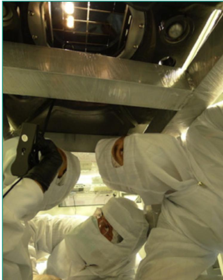
Fig. 1: IFAE engineers assembling the PAUCam astronomical camera in IFAE's clean room, which occupies 44 m<sup>2</sup> in 3 rooms: class 1000 / 10000 / 100000.
