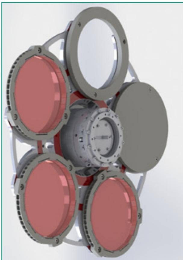
**Fig. 1:** The Filter Wheel Assembly (FWA) of the NISP Instrument. One can see the three filters, the open and closed position and the Cryomechanism installed in the center of the wheel.
