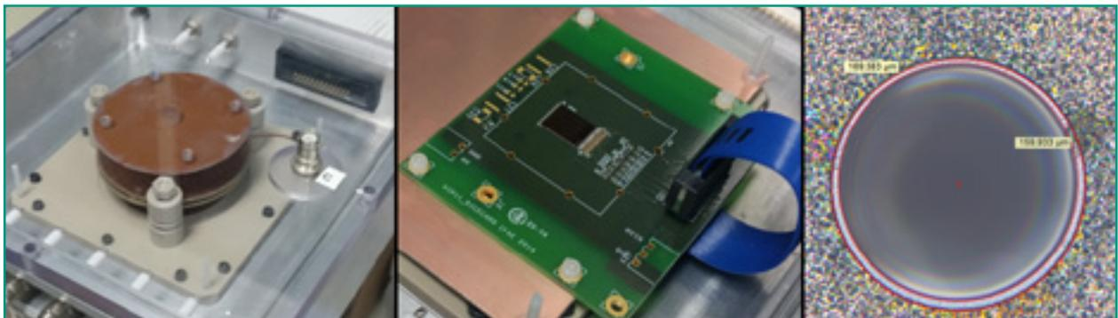
**Fig. 8: (Left) The test chamber. (Middle) Installation of the VIP chip in the detector for first tests. (Right) Photo of the hole of one of the samples. One can see the surrounding aluminum, the "rim", an area around the hole without metal, and the hole. The hole diameter is 80  $\mu\text{m}$ .**
