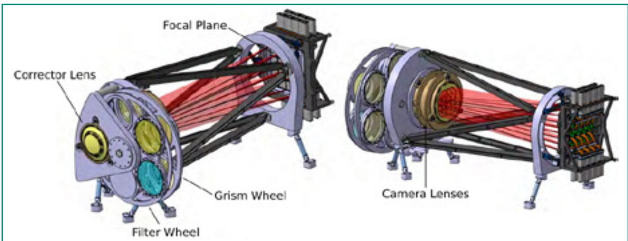
Fig. 2: Artistic view of the NISP Instrument. The FWA is mounted in front and select the filter that its positioned in the light path coming from the mirror before being detected in the Focal Plane
