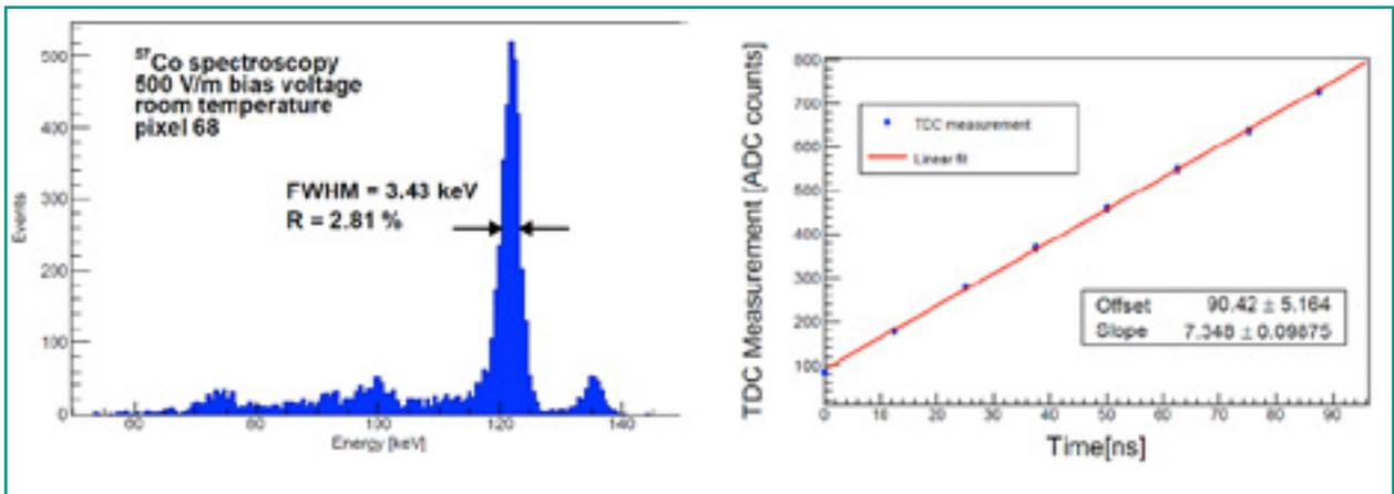
Fig 2: On the left hand side, one can see the spectroscopy of <sup>57</sup>Co and the clear separation of the two peaks at 122keV and 136keV. On the right hand side one can TDC response for various predefine Δt values. The sensitivity is 0.Insec/bit and the overall timing resolution is 1nsec.
