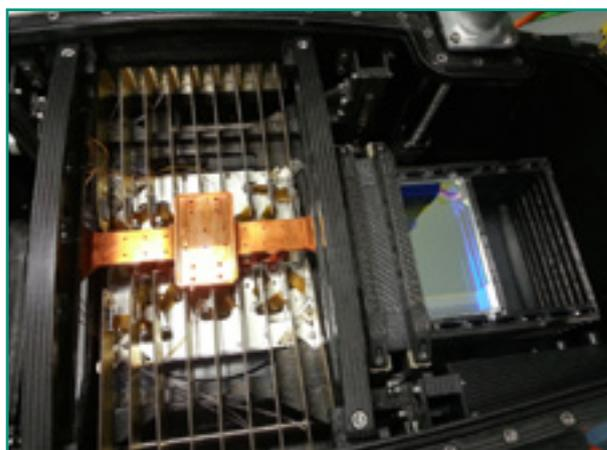
**Fig. 3:** A photograph of PAUCam being assembled. The focal plane will be mounted on top of the Copper cross clearly visible in the photograph. On the right one can see the filter trays (of that side). The long screws are part of the system that moves the trays.
