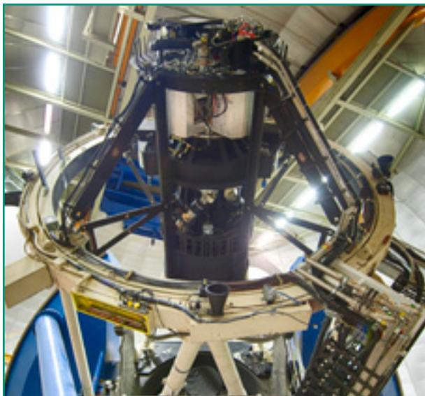
Fig. 1: The complete DES camera, DECam, installed at the prime focus of the Víctor M. Blanco telescope at the Cerro Tololo Interamerican Observatory (CTIO) in Chile.
