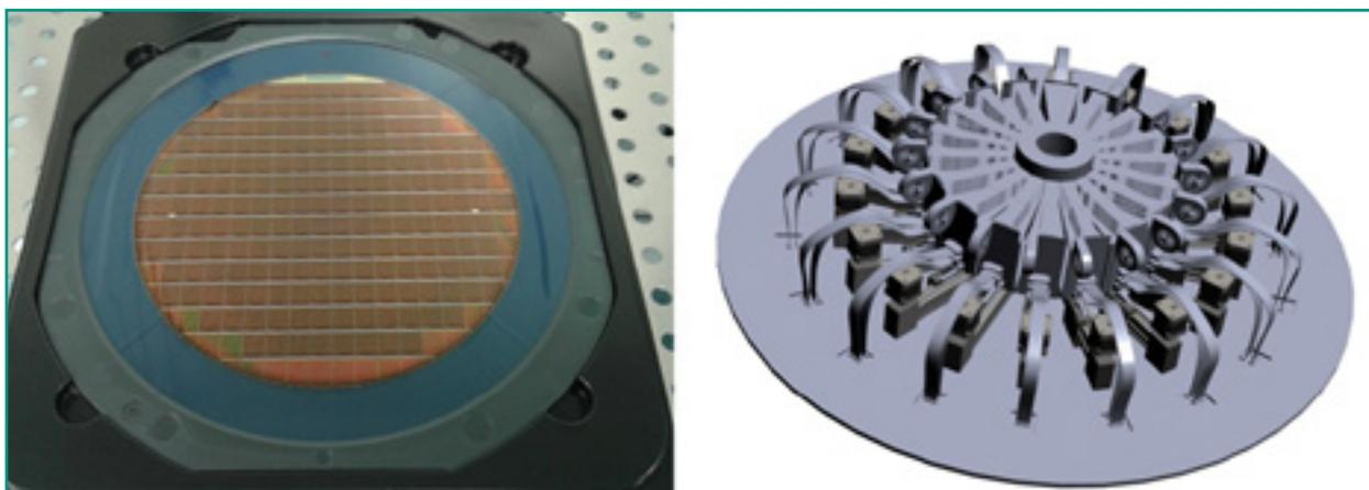
**Fig 1:** On the left hand side one can see the VIP wafer on dice tape. On the right hand side one can see the schematic of VIP PET ring with 18 VIP modules
