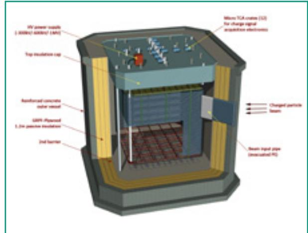
Fig. 6: Schematic representation of the TPC inside the cryostat. The inner detector has dimensions of 6x6x6m<sup>3</sup>.
